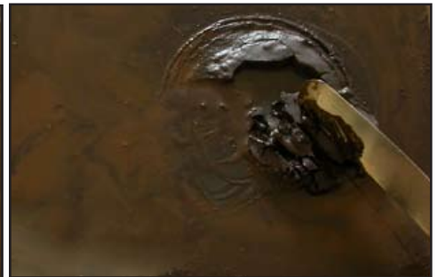
5. Cut into the dried lump of paint.
