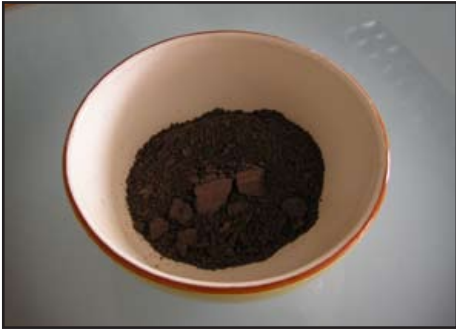
1. Measure about 100 grams or 3 1/2 ounces of glass paint into the mixing bowl
