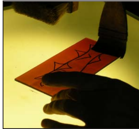
14. How to paint a wash on top of unfired traced lines
