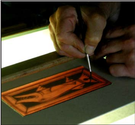
6. Good ways to use the painting bridge (look at the left hand)
